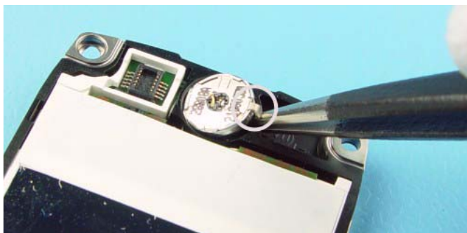
The Speaker is attached with double-sided adhesive Foam Tape. Always use a new tape when mounting the Speaker.
