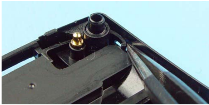
The Power Key has to be unlocked on the lower side first.
