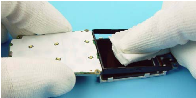
Take a clean cloth and press the LCD from the LCD Frame.
