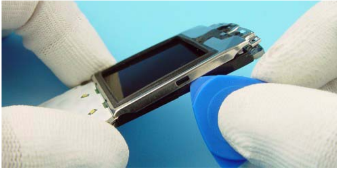
Open the snaps with SRT-6 on both sides of the Display Shield.
