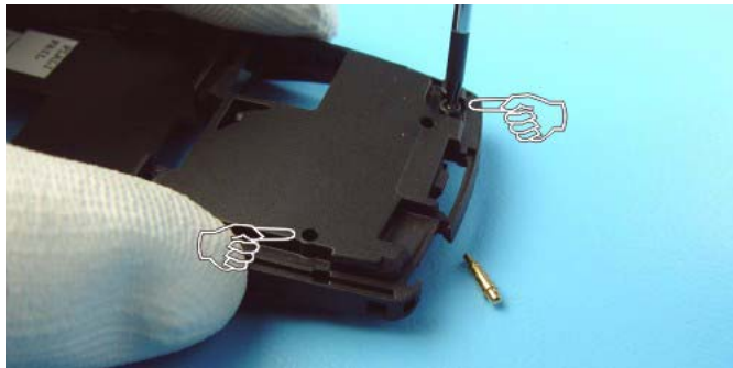
Antenna Pogo Pins can be removed by pushing with Torx driver through the C-Cover.
