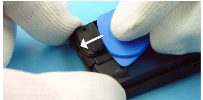
If there is a need to change the Release Button, also SRT-6 can be used.
